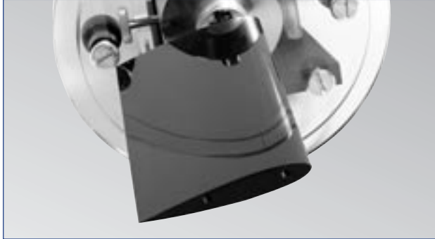
C15-20 Lift & Drag Aerofoil shown fixed to the C15-13 Lift & Drag Balance
