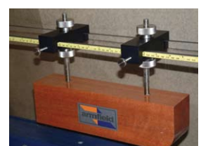
C4-62 Culvert fitting, one edge square, one rounded
