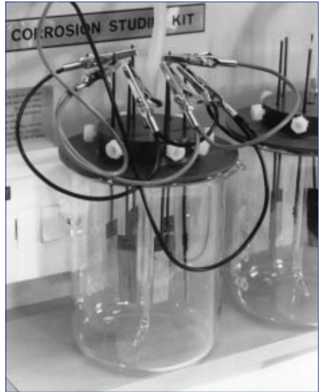
Detail of a single corrosion cell
