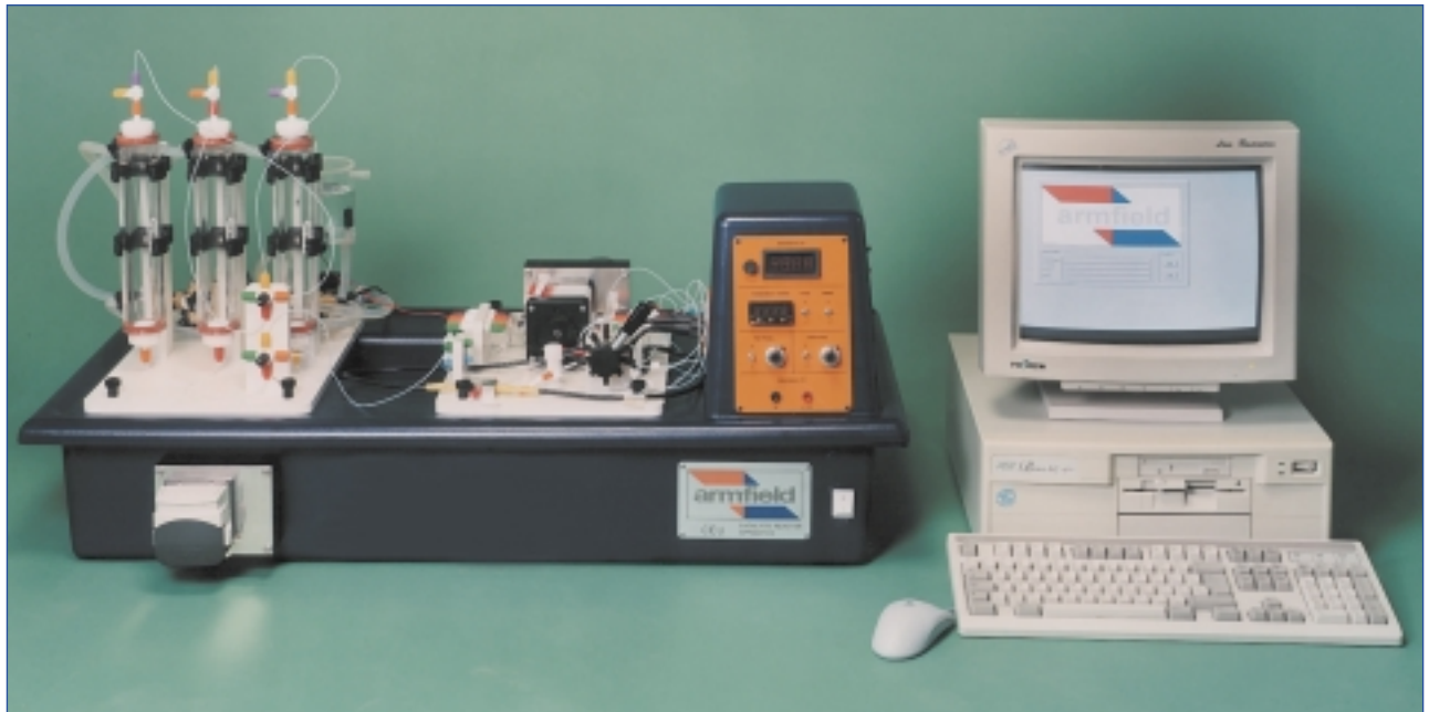
CEU unit shown with the optional enzymic reactor and Flow Injection Analysis (FIA) system.
