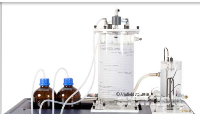
CET-MkII Tubular reactor fitted to CEXC service unit
