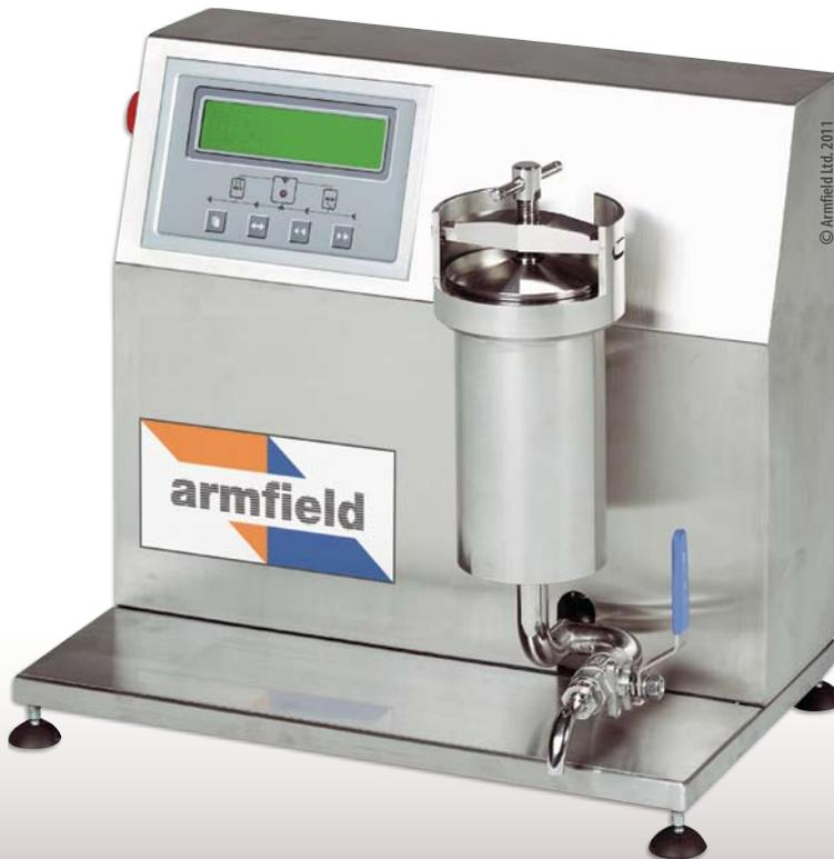
The Armfield FT110 Benchtop Rapid Extractor is used to extract the active constituents from small (1 litre) samples of materials.
