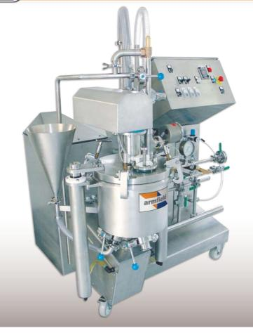
The new Armfield FT141 and FT142 are versatile batch processing vessels, the FT142 having UHT capability. They are suitable for high shear mixing, dispersing, homogenising, emulsifying, evaporation and vacuum de-aerating.
