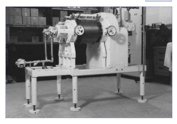
The Armfield Drum Drier consists of a nip fed twin cylinder drying machine, cast from Meehanite GA, cast-iron with combined endplates and trunnions. The rolls are accurately ground on the circumference, bored internally to ensure even heat transference, and suitable for working with steam at up to 5.5 bar. The rolls are carried in grease lubricated bearings which are housed in circular endplates mounted on the base plate of the machine.
