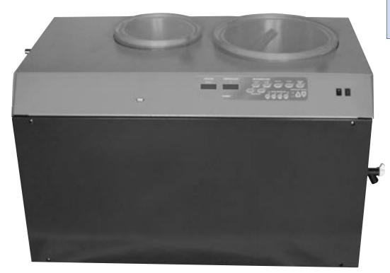
The Armfield Freeze Drier is a compactly designed unit with an insulated working chamber 300mm diameter x 385mm deep. It incorpoates a built in refrigeration system and temperature controlled heating system. With the working chamber and condenser chamber constructed from stainless steel, it offers excellent corrosion resistance and can be easily sterilised.
