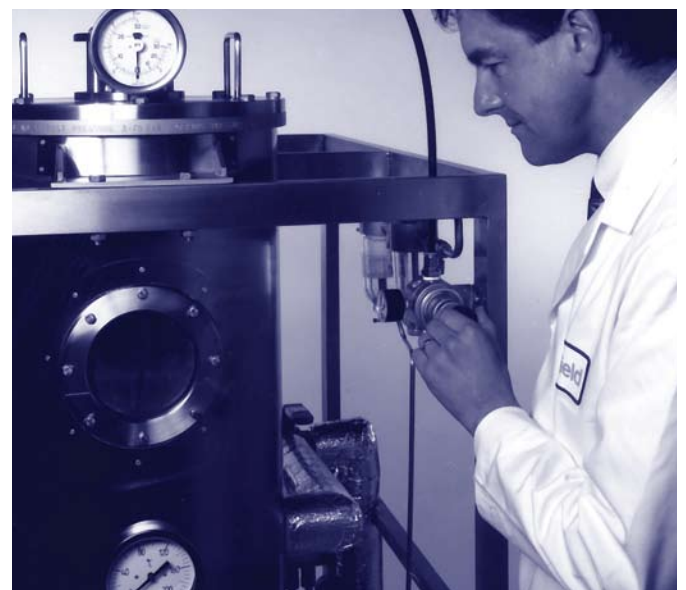
Adjusting the rotational speed of the turbine agitator air motor
