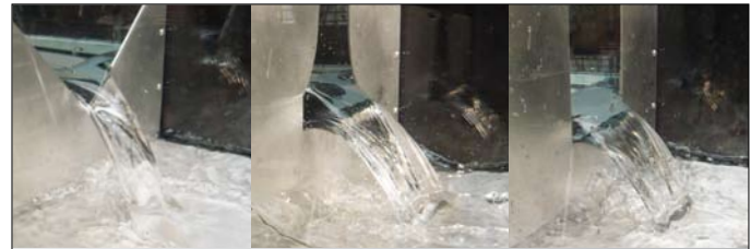
V-notch, Sutro and Rectangular plate weirs Trapezoidal and Sharp Crested weirs also included with the S6-20.
