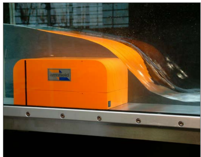
S6-21: Broad crested weir - in operation
