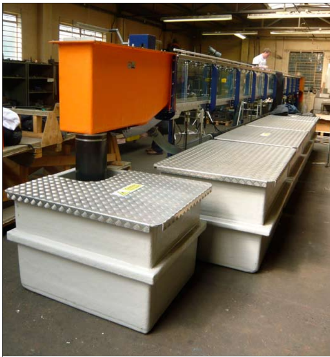
S6MkII view from outflow end showing sump tank arrangement
