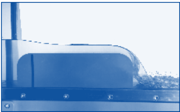
S6-21: Broad crested weir - in operation (above) and theory (right)
