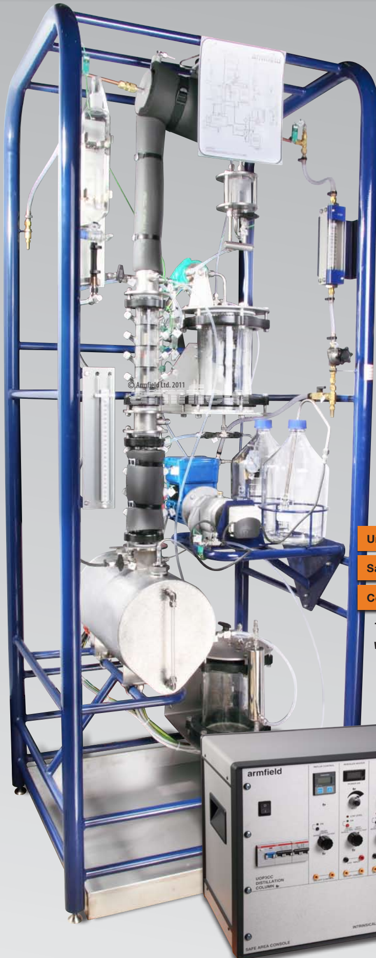
Above: Computer interfaced distillation column UOP3CC shown with safe area console
