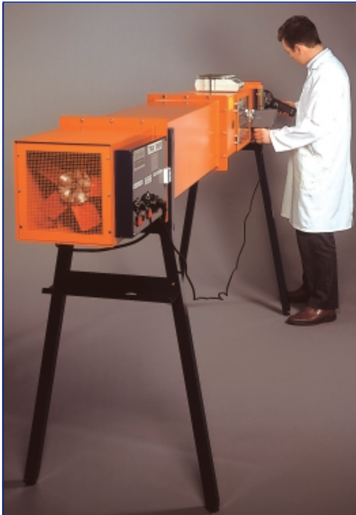
The UOP8 Tray Drier with operator using psychrometer downstream of sample trays.
